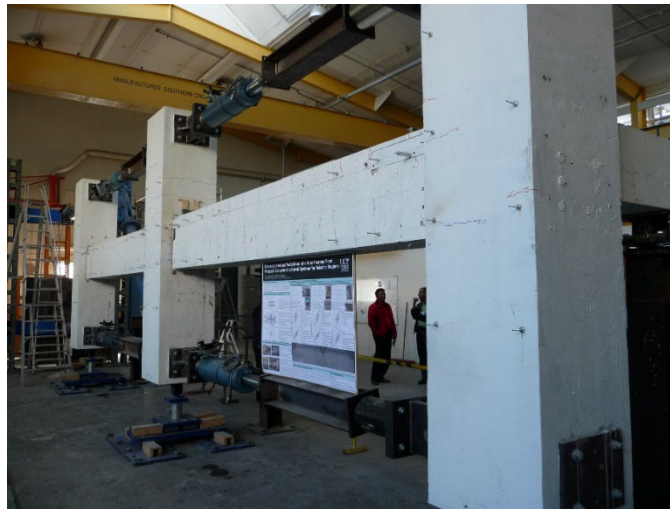
Figure 1. Full-scale reinforced concrete columns and beams being tested in a laboratory.
