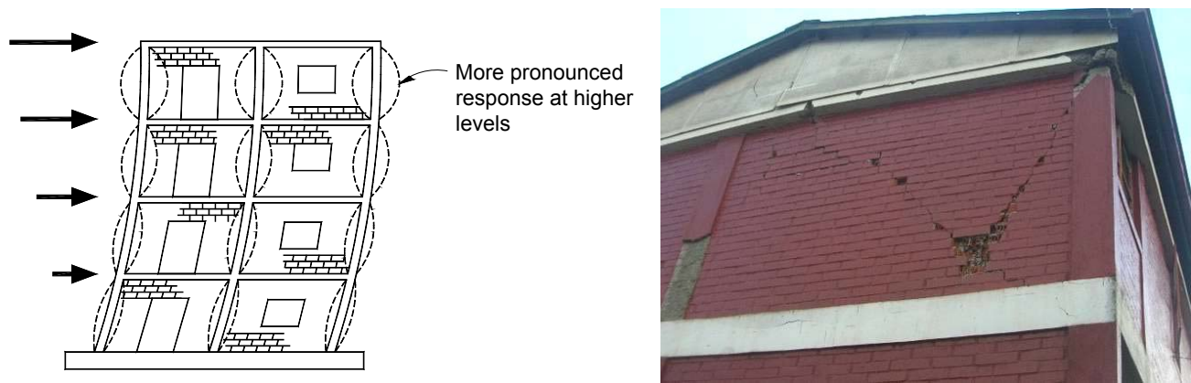
Figure 15. Out-of-plane seismic response of confined masonry walls: a) a mechanism of seismic response (Tomazevic, 1999, and b) observed damage at the top floor level of a building after the 2010 Maule, Chile earthquake (M. Astroza).
