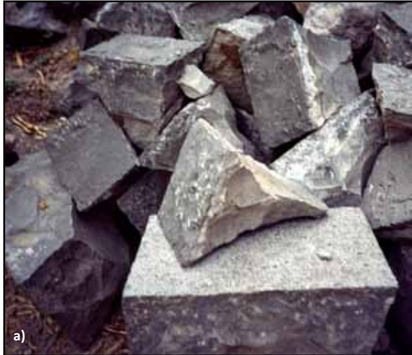
Figure 1.21 Semi-dressed stones ready for wall construction: a) wedged stones in Maharashtra, India (photo: S. Brzev), and b) shaped stones in Pakistan (photo: T. Schacher)
