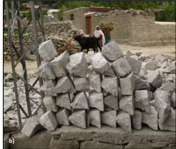
Figure 1.21 Semi-dressed stones ready for wall construction: a) wedged stones in Maharashtra, India (photo: S. Brzev), and b) shaped stones in Pakistan (photo: T. Schacher)
