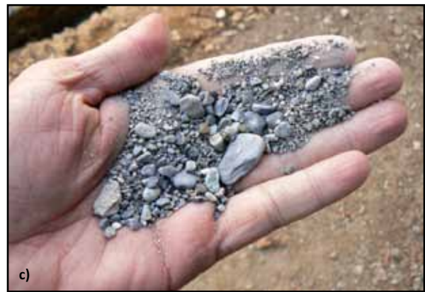
Figure 3.42 Sand for different uses: a) fine sand for plaster construction; b) coarse sand for mortar and concrete construction, and c) excessively coarse sand (photos: Smart Shelter Foundation)
