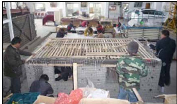
Figure 4.26 Testing polypropylene bands at IEM in Harbin, China (photo: W. Feng)
