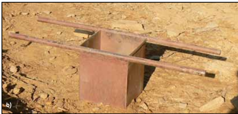
Figure 3.45 Measuring concrete materials: a) proportioning concrete ingredients using a measuring box, and b) a measuring box (photos: Smart Shelter Foundation)
