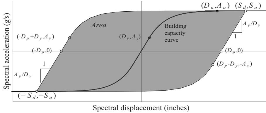
**Figure 4.** Establishing effective damping ratio at HAZUS-MH performance point.
