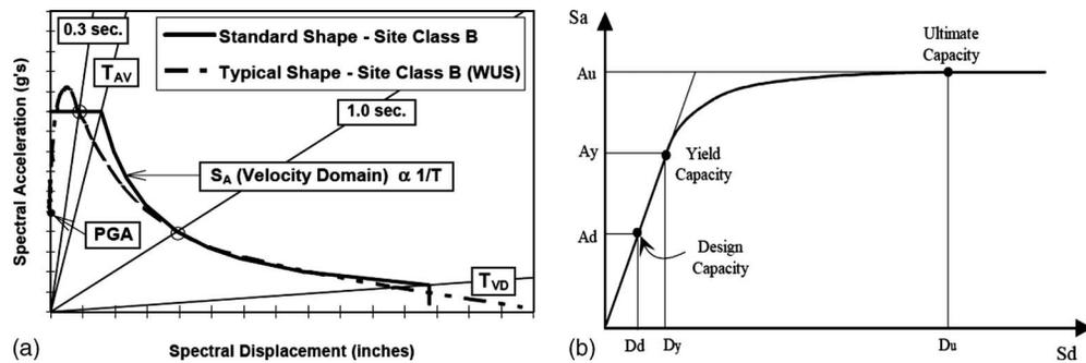
**Figure 2.** HAZUS-MH standardized response spectrum shape and capacity curve (NIBS and FEMA 2003 Figures 4b and 5d).
