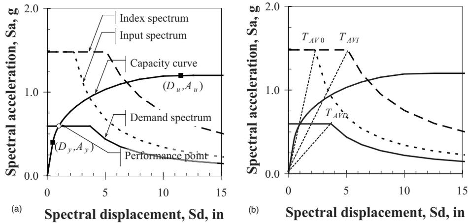
**Figure 3.** HAZUS-MH capacity curve and various response spectra used here (a), and corner periods used here (b).
