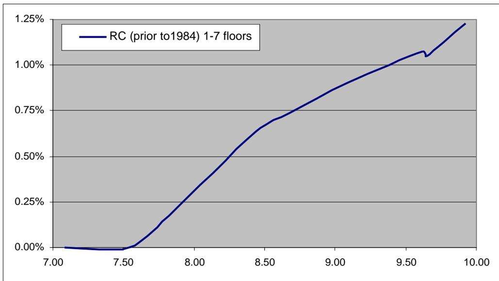
Figure 4 Estimation of collapse probability for RC buildings with respect to the level of seismic intensity using the neighborhood level data from the 1986 Kalamata earthquake
