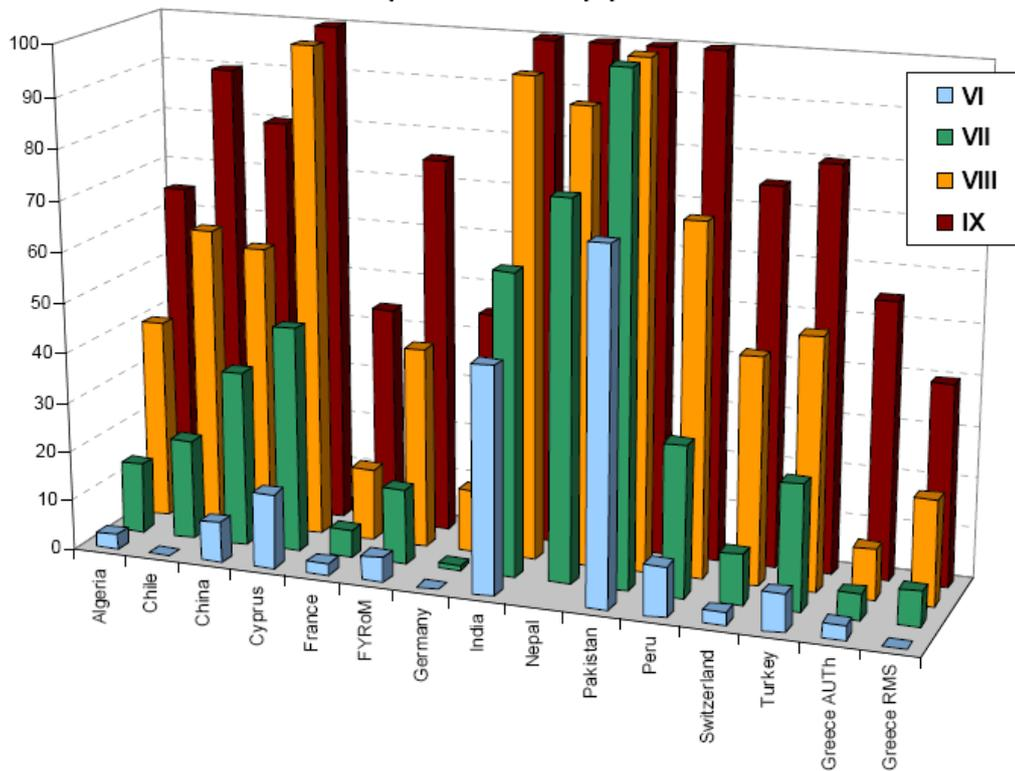
Figure 6 Collapse probabilities in the intensity range VI to IX for unreinforced stone masonry buildings as provided by the experts solicited by EERI in various countries.
