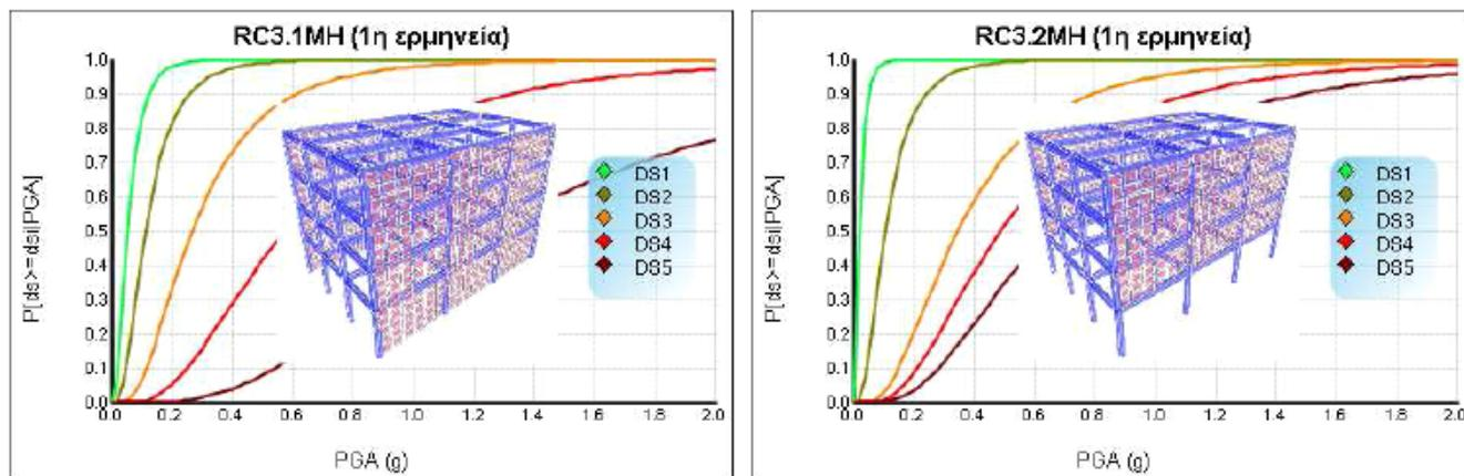
Figure 5 Seismic vulnerability curves for medium-rise RC frame buildings with brick-infill (left) and with pilotis (right) designed according to the latest seismic codes (NEAK/EAK 2000).
