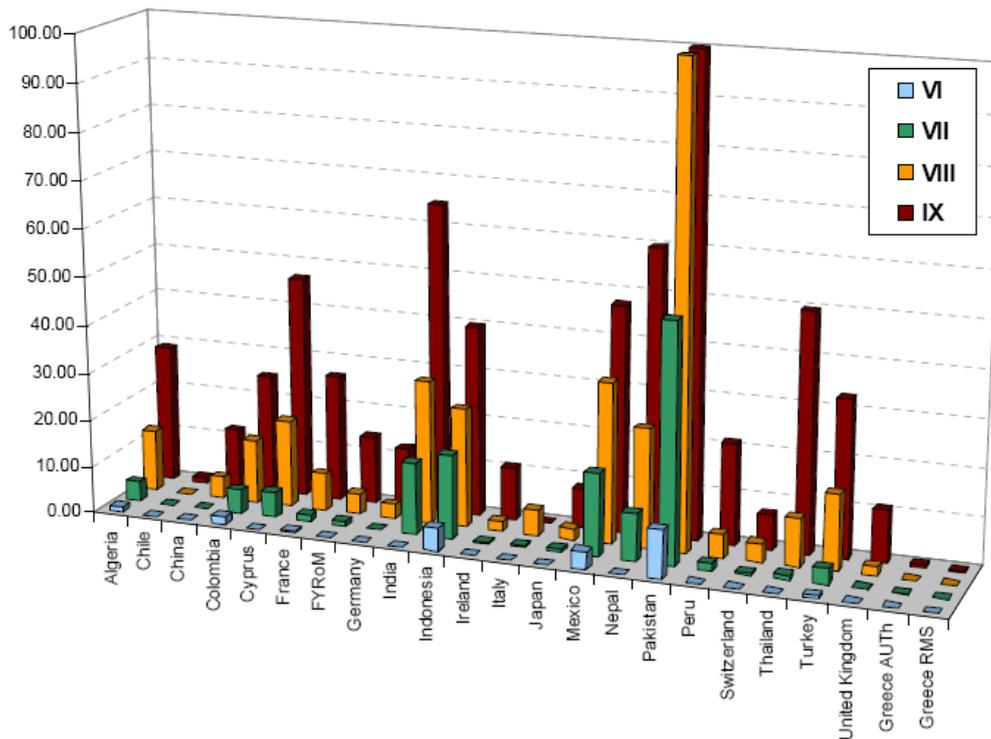
Figure 7 Collapse probabilities in the intensity range VI to IX for reinforced concrete buildings as provided by the experts solicited by EERI in various countries.
