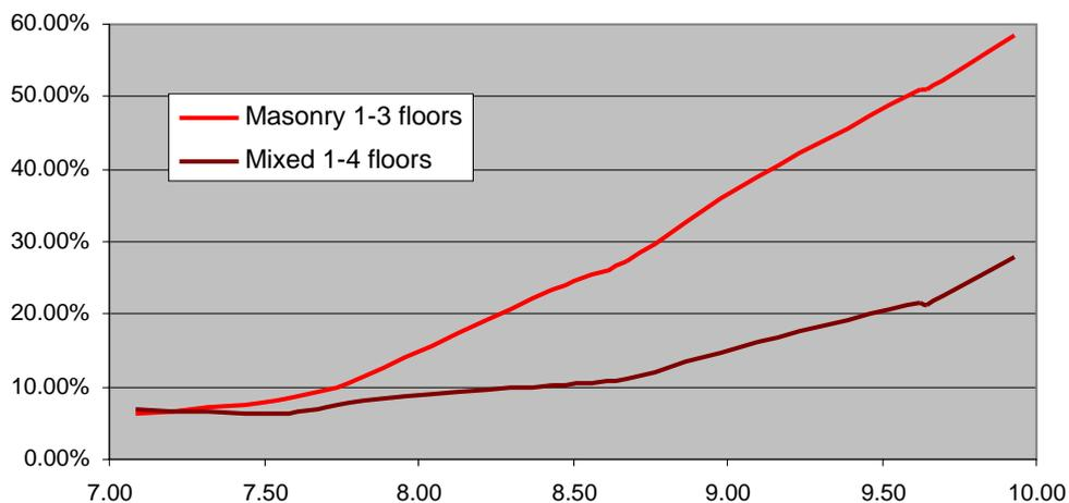
Figure 3 Estimation of collapse probability for URM and mixed URM+RC buildings with respect to the level of seismic intensity using the neighborhood level data from the 1986 Kalamata earthquake
