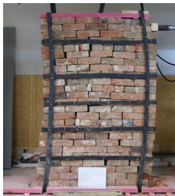
Figure A.4 Walls 1 (left) and 2 at a similar stage of their cyclic loading sequence.
