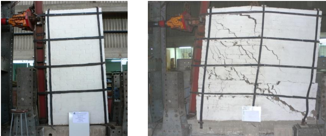
Figure A.7 Horizontal load is applied to the top of a vertical steel post pin-jointed at its base which then transfers loads to the wall in compression, via wooden blocks, and tension, via horizontal straps. The 1.2 m long wall (left) is being pulled to the left and is rocking at its base while the 2.4 m long wall (right) has undergone five cycles of loading.
