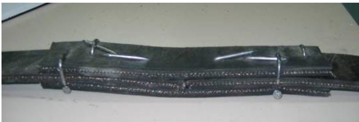
Figure A.1 A completed nailed joint showing the bent nails.
