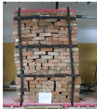
Figure A.4 Walls 1 (left) and 2 at a similar stage of their cyclic loading sequence.
