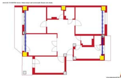
Figure 3B: Plan of a Typical Building (after the retrofit)- the jacketed columns are yellow-colored
