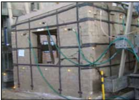
Figure 4.15 Shake table testing of an adobe building model reinforced with tire straps
