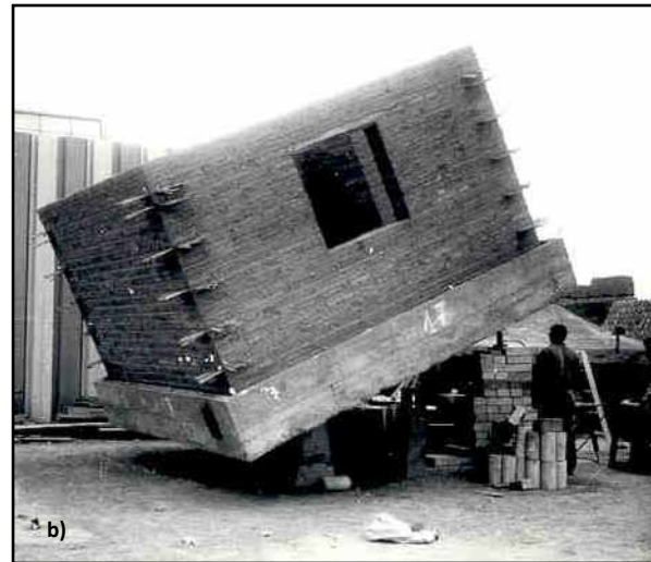
Figure 4.2 Seismic performance of an unreinforced and a strengthened adobe building: a) Unreinforced specimen, and b) Specimen with cane reinforcement (Blondet et al. 2002)
