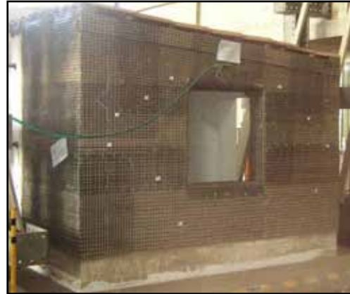
Figure 4.10 Reinforced adobe house with geomesh during a shake table test at the PUCP.
