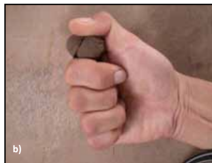
Figure 3.1 Dry strength test: a) Adequate soil, and b) Inadequate soil
