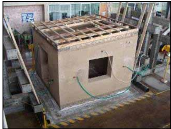
Figure 4.13 Adobe model reinforced with geomesh and covered with mud plaster during the shake table test (source: Bossio 2010)
