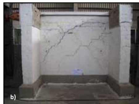
Figure 5.3 Repairing seismic cracks on adobe buildings at PUCP: a) Crack injection on adobe module, and b) Repaired module being tested
