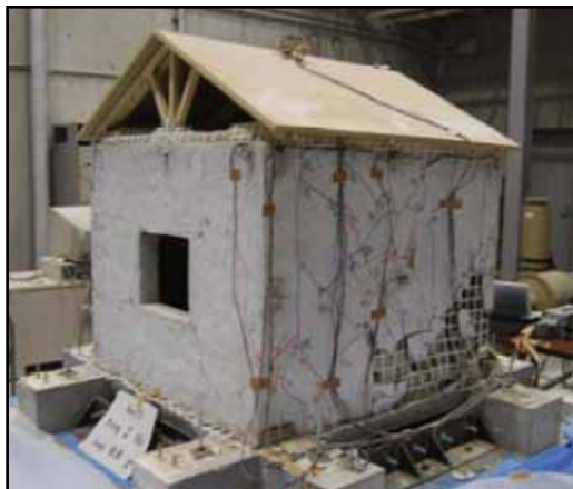
Figure 4.16 Full-scale adobe model reinforced with PP-bands after a shake table test
