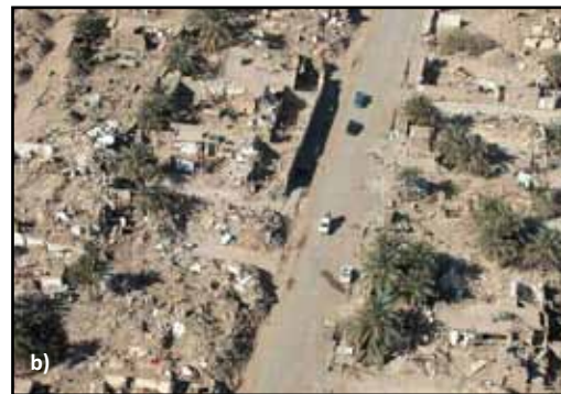
Figure 2.1 Collapsed adobe buildings: a) 2001 El Salvador earthquake (photo: D. Dowling), and b) 2003 Bam, Iran, earthquake (source: Mehraïn and Naeim 2004)
