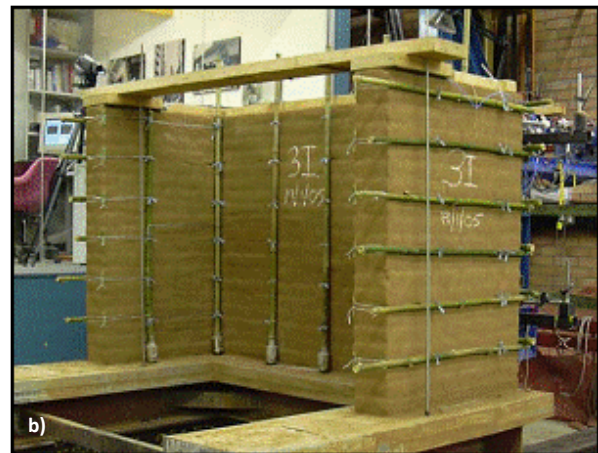
Figure 4.7 Adobe building models with external bamboo: a) Vertical bamboo on both sides, and b) Vertical and horizontal bamboo
