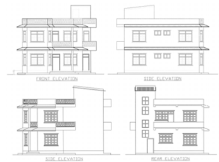
Typical elevations of a RC frame residential house
