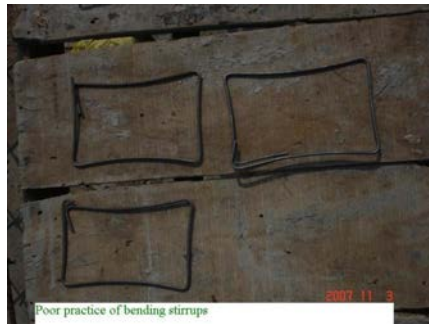
Poor practice of bending stirrups Defective stirrups due to 90 degree bends
