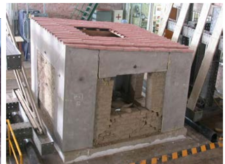
Fig. 32: Model tested in PUCP shaking table, with some damage under severe earthquake.
