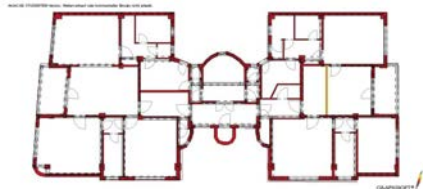
Figure 11: Architectural plan of a current floor (after Bostenaru(2004)). Yellow marks new partition walls.
