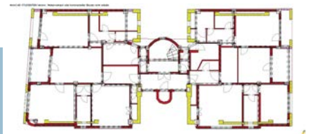
Figure 38: Retrofit plan for the typical building considered, using shear walls and column jacketing. The retrofit elements are highlighted. (from Bostenaru(2004))
