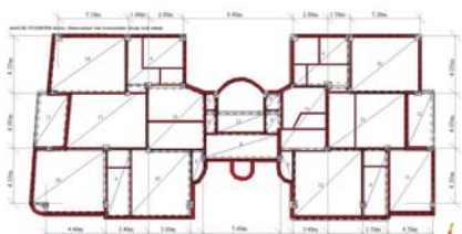
Figure 17: Floor plan including the load bearing elements as masonry walls and slab thickness (blue), as well as the spans. (after Bostenaru(2004))
