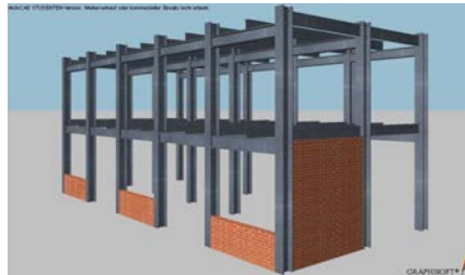
Figure 21: Key seismic features: infill walls (an archive photo showing infilling of metal frame on the building site is found in N
