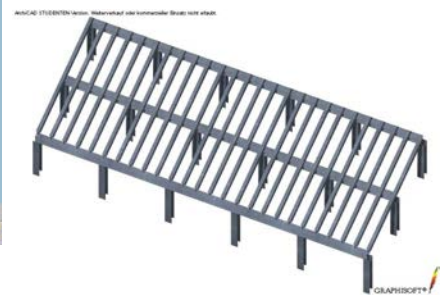
Figure 13: Axonometric view of key load bearing elements in variant 1
