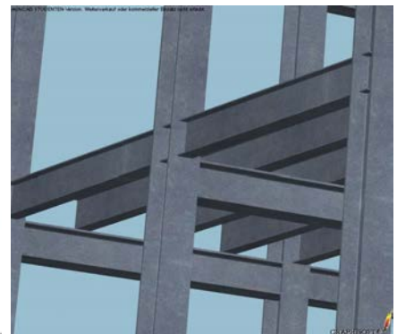
Figure 16: Critical structural detail: column-joint connection (an archive photo of such a structure in Kassel-Rothenberg, architect Otto Haesler, can be seen in Stein Holz Eisen 1929)
