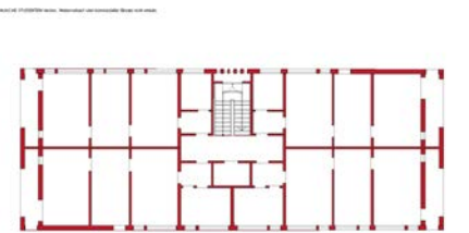
Figure 26: Layout of load bearing walls and their openings in a current floor
