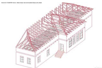
Figure 22: Axonometric view showing the roof
